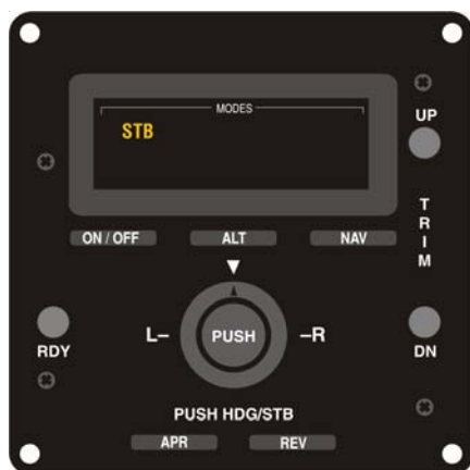
Fig. 2-17. AP Display, STB Mode Engaged (System Fifty)
