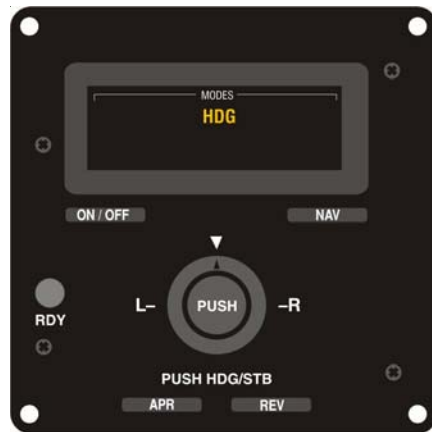
Fig. 2-6. AP Display, HDG Mode Engaged (System Forty)
