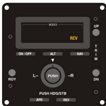
Fig. 2-21. AP Display, REV Mode Engaged (System Fifty)
