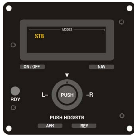
Fig. 2-5. AP Display, STB Mode Engaged (System Forty)
