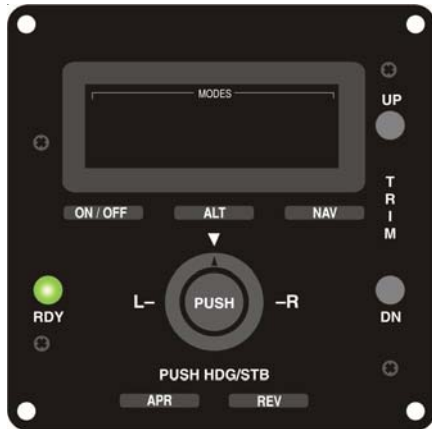
Fig. 2-15. AP Display, RDY for Operation (System Fifty)
