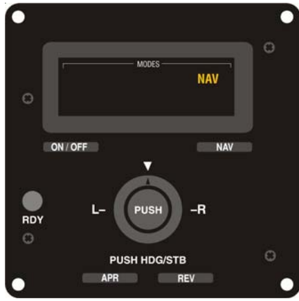
Fig. 2-7. AP Display, NAV Mode Engaged (System Forty)
