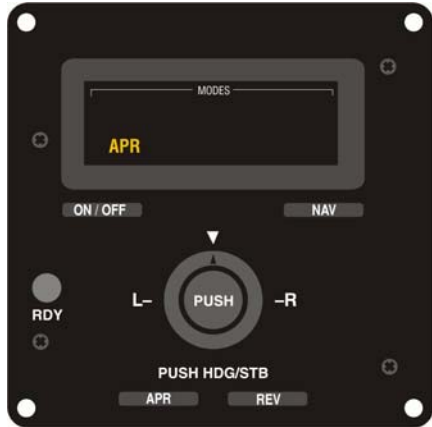
Fig. 2-8. AP Display, APR Mode Engaged (System Forty)
