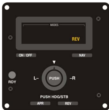
Fig. 2-9. AP Display, REV Mode Engaged (System Forty)
