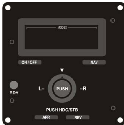
Fig. 2-4. AP Display, Turn Coordinator Failure, RDY Lamp Does Not Re-Illuminate (System Forty)
