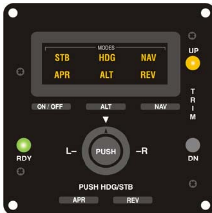
Fig. 2-13. AP Display, TRIM DN Lamp Extinguished (System Fifty)
