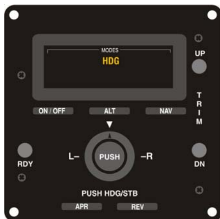
Fig. 2-18. AP Display, HDG Mode Engaged (System Fifty)
